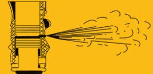
**Note:** Water can build up in the combustion chamber from rain or condensation. If not removed, this water can be forced up the injector & into the fuel pump or even the fuel tank. Water is the main source of downtime on a diesel hammer. Blow out your hammer each morning. Failure to do so will result in hard starting & irregular stroke. Never dry fire a hammer to remove unwanted water or oil.
